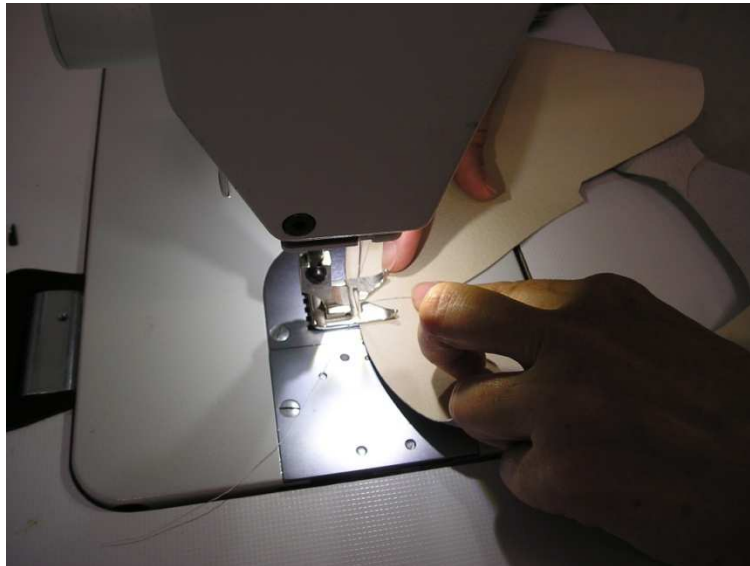
Picture 27 Zig –zag stitching save material-this is possible to use at some connections
