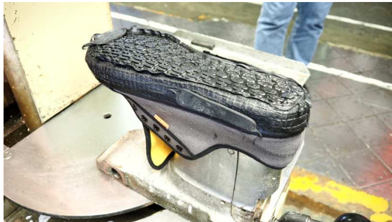
Picture 16 Correction of the places where material was missing
