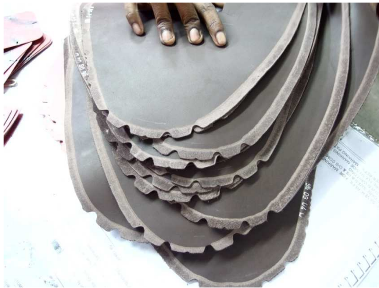
Picture 6 Example of good design of „V“ notches and leader grain skiving
