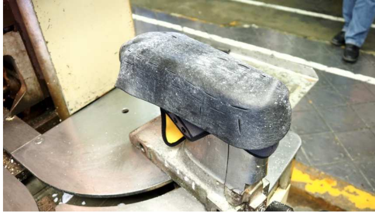
Picture 14 Upper with 2 layers of rubber ready to be inserted for the first dressing
