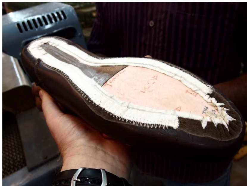
Picture 5 „V“ notches will help folding of the material in front area
